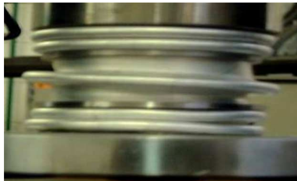
Fig. 5. Typical example of a fully crushed 3-level subdivided aluminum structure deformed by axisymmetric mode.
